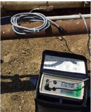
**Figure 3.** Ultrasonic (Doppler) flowmeter.
