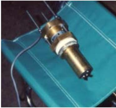
**Figure 4.** Turbine flowmeter.
