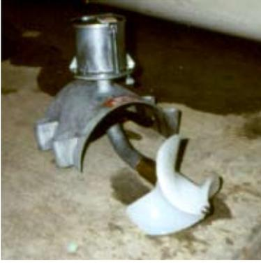
**Figure 1.** Propeller flowmeter.
