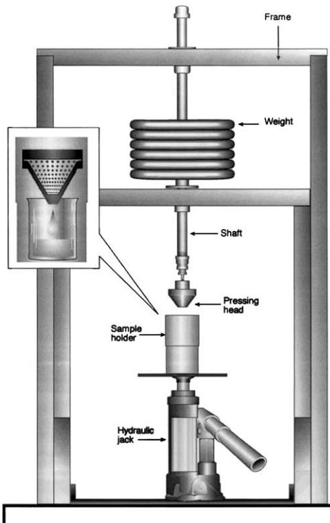
Fig. 1. Scheme of the pressing apparatus.
